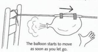
Air is forced out of the balloon in one direction.
